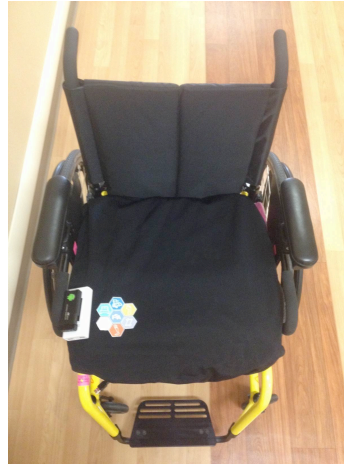
Figure 1: Wireless pressure mat shown placed over a seat cushion with portable power and mini-PC shown
